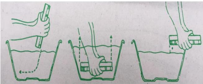
Holding frame tightly dip it into the tray, pausing at the bottom. Then take it out but hold on an angle to drip and remove excess water.
