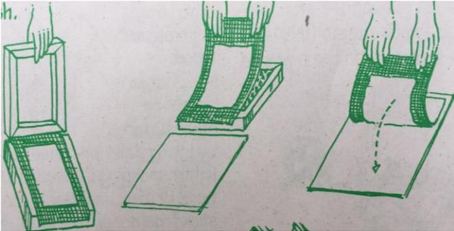
With drying board ready, peel the mesh off the screen. Then slowly lower the mesh down onto a drying board. Sponge the mesh and then peel the mesh off leaving the paper behind to dry.
