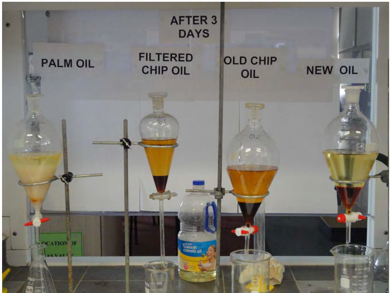
Figure 8 All four biodiesel samples after 3 days. It can be seen that the dbiodiesel produced from palm oil has taken much longer to separate out. It also can be seen that the old chip oil (unfiltered) contains particulate matter.
