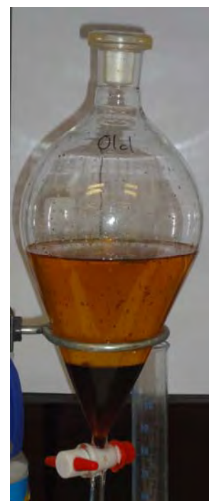
Figure 7 The biodiesel (top layer) produced from unfiltered fish and chip oil – viewed after 3 days
