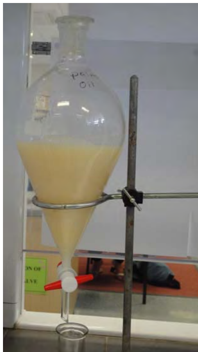
Figure 3 The initial mixture of palm oil, methanol and potassium hydroxide, just after shaking
