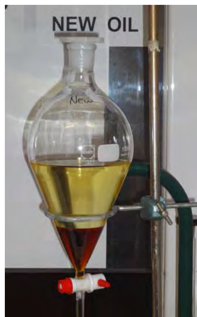
Figure 5 The biodiesel (top layer) produced from fresh canola oil – viewed after 3 days
