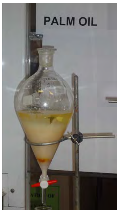
Figure 6 The biodiesel (top layer) produced from palm oil – viewed after 3 days
