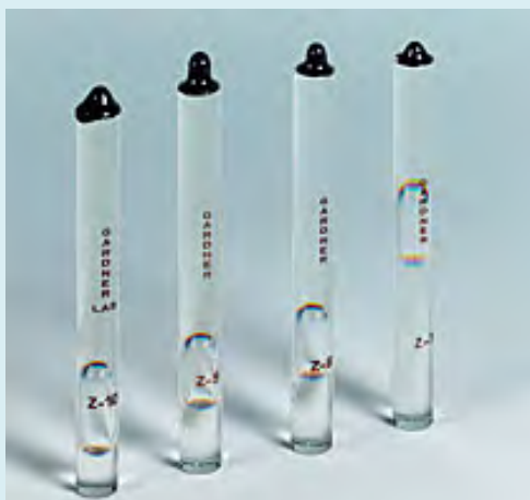
Figure 1 A set of bubble viscometers containing different oils
