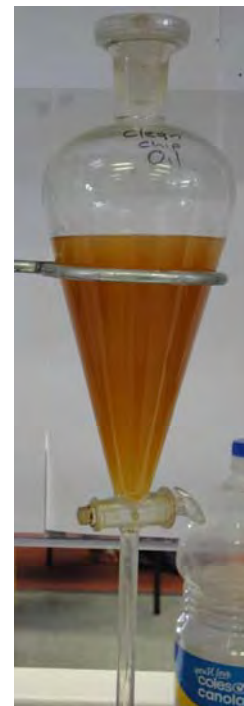
Figure 4 The initial mixture of filtered fish and chip oil, methanol and potassium hydroxide, just after shaking.
