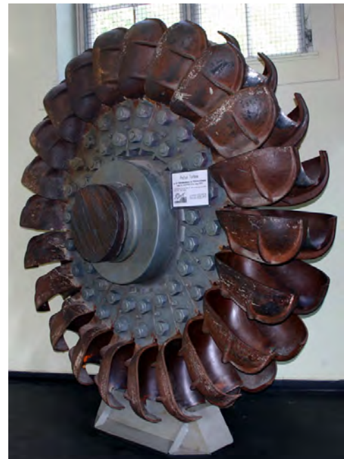
A Pelton wheel from the Walchensee Power Plant, Germany. Credit: Wikimedia Commons
