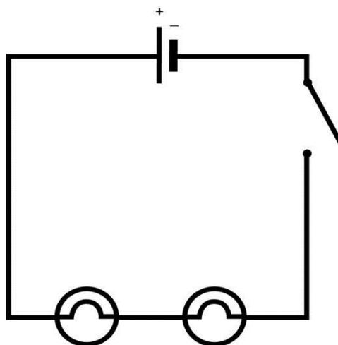
Figure 2: The circuit diagram of the series circuit
