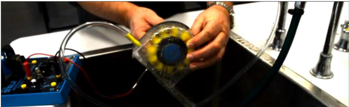
The Pelton wheel set-up – do this over a sink.
