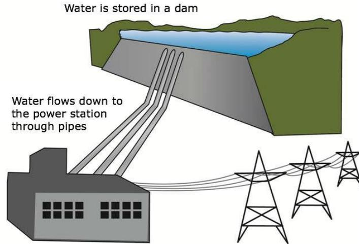
In the power station the water is used to push giant turbines. These in turn cause huge wire coils to spin inside giant magnets, which generates electricity
