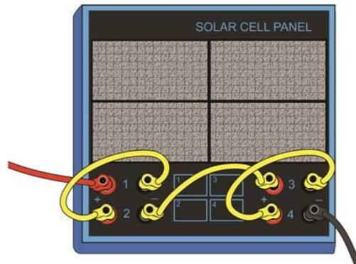
Figure 5: Connecting Cell 3 to Cell 4
