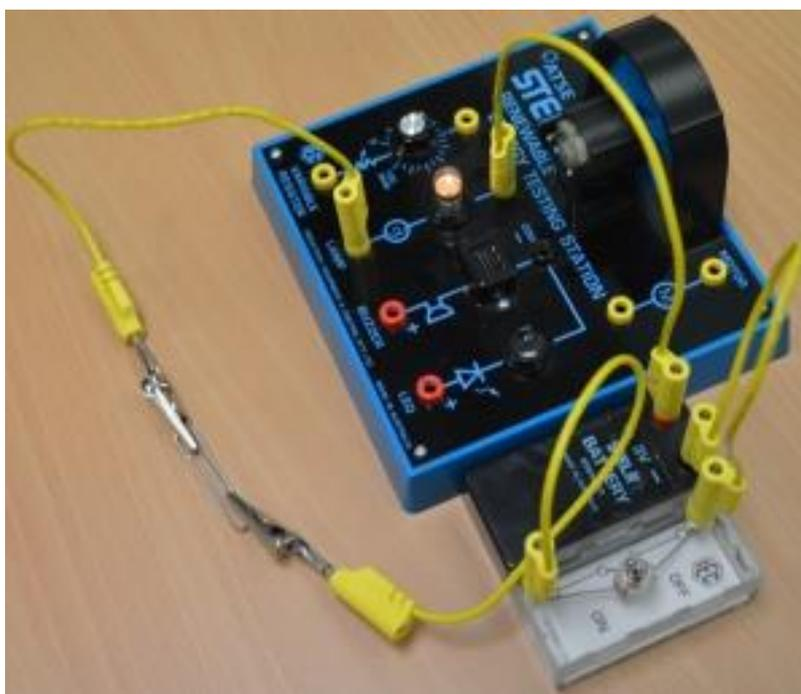
One way to test if a material is a conductor or an insulator
