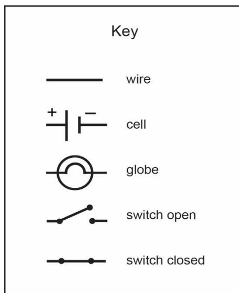
To make circuit diagrams as clear as possible they are always drawn with connecting wires in a square or rectangle.
