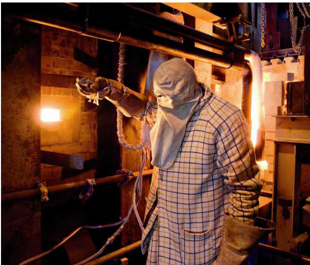
Figure 2 Manufacturing glass. Sand and limestone are two of the main raw materials used to make glass. These and the other raw materials required for the particular type of glass being manufactured are heated together in a furnace to over 1000 °C. The fuel burnt to produce this heat energy is usually natural gas.
