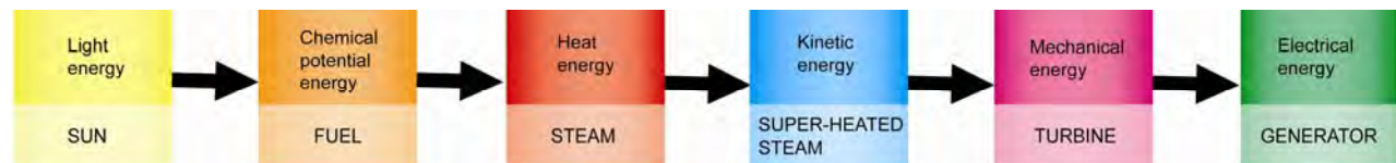
Figure 4 The main energy transformations that occur when electricity is generated at a coal-fired power station
