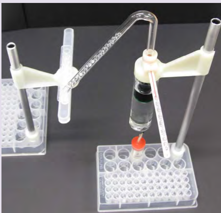
Figure 3 This is the micro-scale distillation equipment you will use. The glass tube sloping downwards is the condenser. On this small scale you don't need the condenser to be cooled by water.
