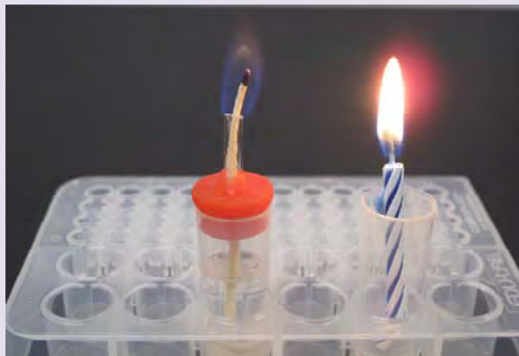
Figure 2 A microburner is about the size of a small birthday candle. Notice that the flame from burning methylated spirits is almost invisible. It is described as a 'clean' flame because unlike a candle flame, it does not create smoke or put black soot on objects above it.
