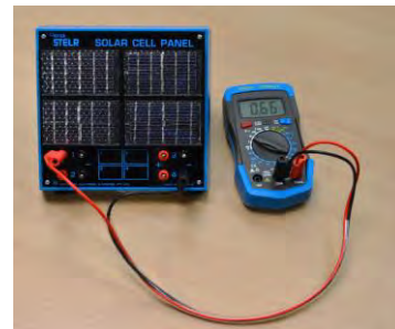
STELR solar panel connected to multimeter
