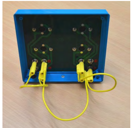
Series connection shown at the back of the panel
