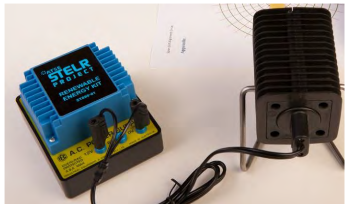
Connect the STELR lamp to the power pack and the power pack to the mains.
